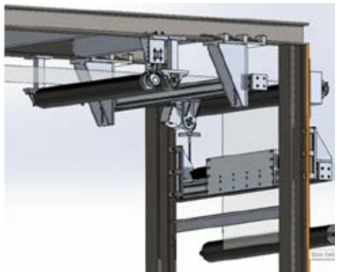
Solid model of the wrinkle detection system designed for the web coater. Source: Vision Optronix/Teledyne Dalsa
