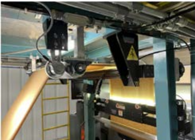
The installed wrinkle detection system in the customer's web coater. Source: Vision Optronix/Teledyne Dalsa
